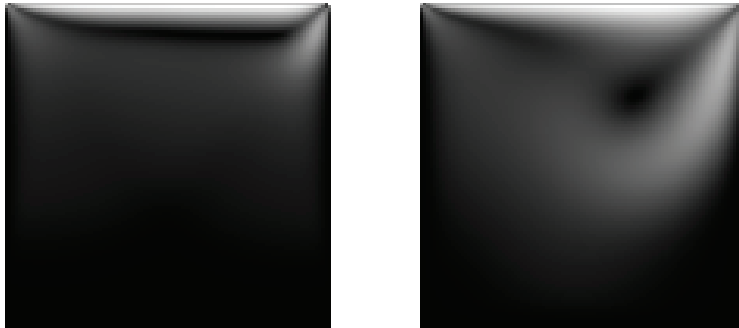
Figure 4: Velocity field of an example 2D lid cavity simulation, iterations 150 (left) and 1000 (right)
